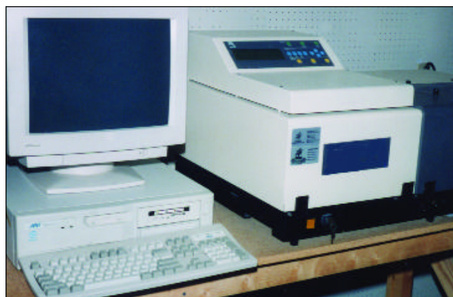
Example of a modern Fourier transform infrared spectrometer Photos courtesy of the author
